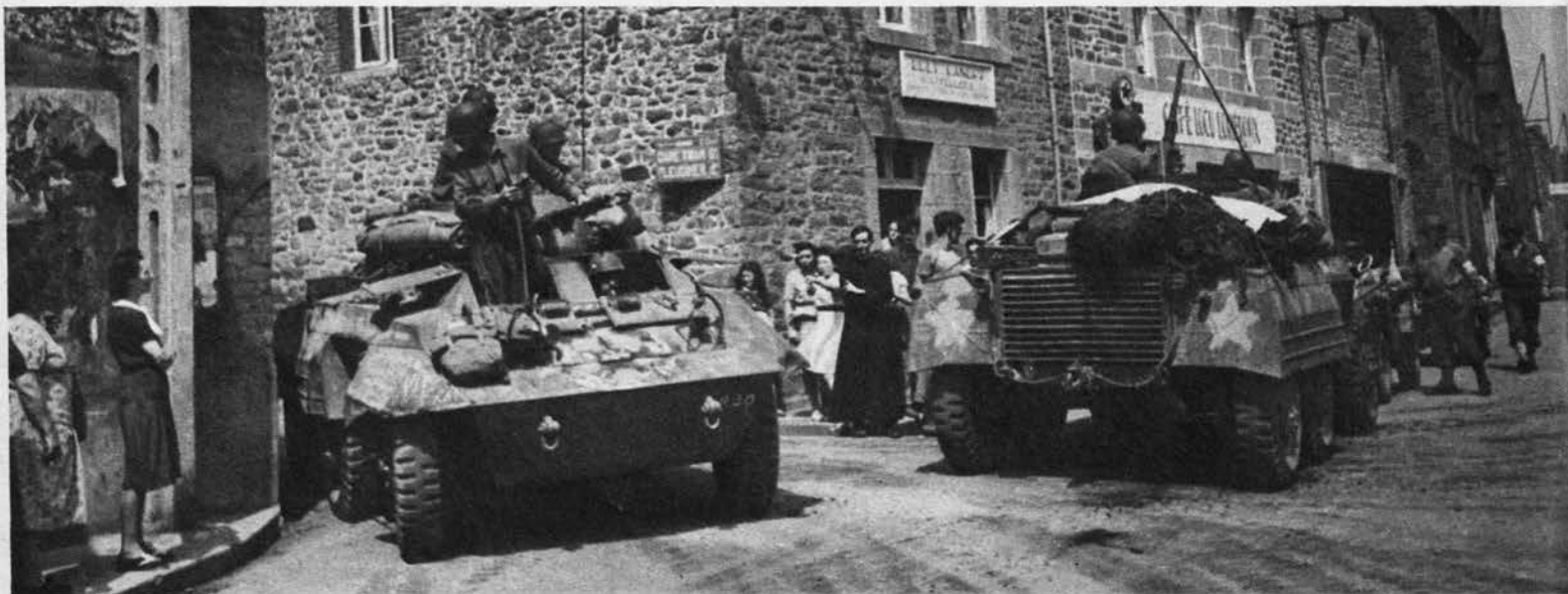
Twin U. S. armored cars tour French town on reconnaissance. They are exactly alike except for armament. The M-8 (left, head-on) has a 37-mm. gun in a round, open-topped turret like that of a light tank.
